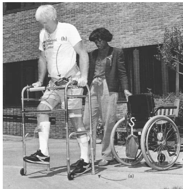
Figure 3 Parastep Electrical Stimulation System developed by Daniel Graupe from the University of Illinois, USA
