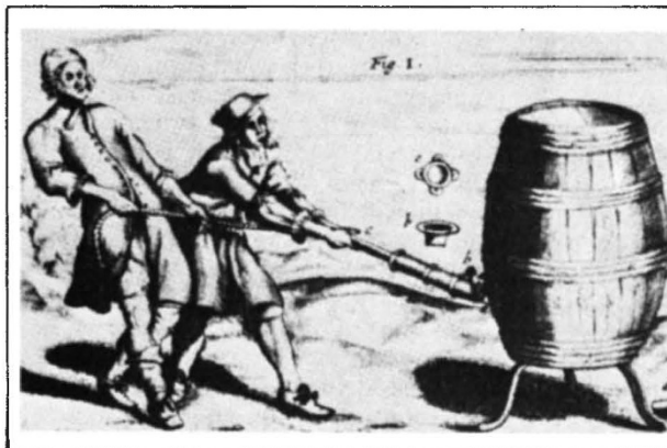
An experiment of Otto von Guericke (1602–1686), a predecessor of Robert Boyle, attempting to produce a vacuum by exhausting a sealed cask filled with water. The illustration is taken from a corrected reprint of A. Rupert Hall's From Galileo to Newton , first published in 1963. The new edition is published by Dover in the United States and Constable in Britain, prices $6, £4.50 respectively (pbk).
