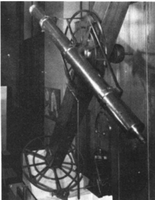
W.H. Smyth's clockwork-driven telescope, 1829
