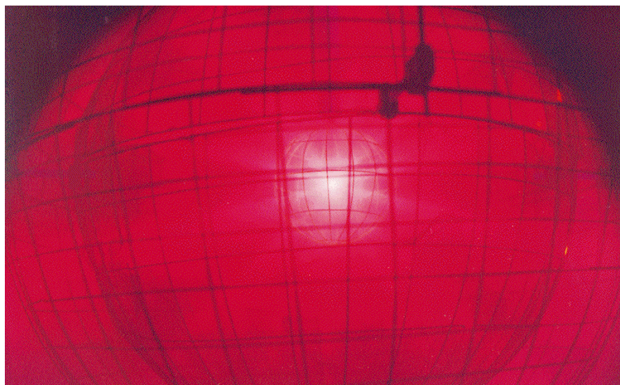
Figure 2 Plasma in an inertial-electrostatic confinement device at the University of Wisconsin. This type of device has provided proof-in-principle that fusion can be produced with D-^3He , a second-generation fuel, at low levels of power input.
