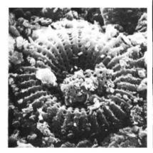
very distinct shapes, some of which are typical of warm sea diatomites with dimensions of about 10  $\mu$ . Debris particles were less than 1  $\mu$ . The figures here show two of the photographs which he obtained with a JSM-U3 scanning electron microscope with a 25 kV electron beam. The magnification was between 3,000 and 10,000.
