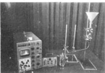
The source of the backscatter is unknown, although Fowlis does point to dust particles or microscopic bubbles as possible candidates; the important practical point, however, is that the system offers a cheap and apparently accurate means of measuring such flow, no matter how the effect works.
