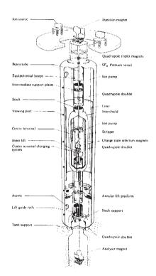
It is planned that the accelerator will be operated in an atmosphere of pure sulphur hexafluoride held at a pressure of several atmospheres to decrease the possibility of electrical breakdown through the gas. One of the chief problems associated with the construction of an accelerator operating at such high voltages is the building of parts capable of withstanding the electrical surges caused by sudden discharges of high voltages.
