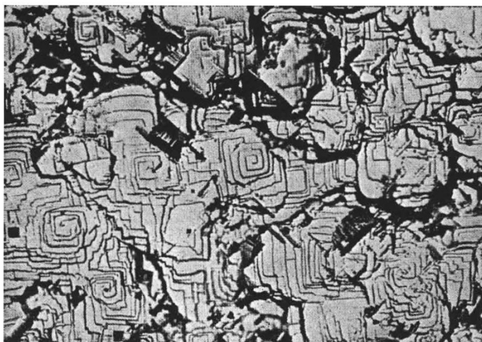
Growth spirals of copper deposited from acid copper sulphate. From Fischer, H., Electrochim. Acta , 2, 50 (1960); reproduced in the second edition of Electrodeposition and Corrosion Processes by J. M. West (Van Nostrand Reinhold, London, 1972; £2.25).
