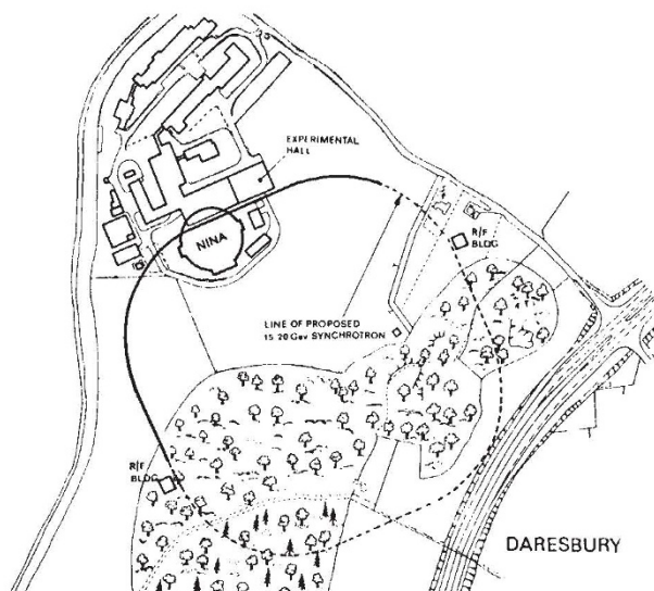
One of the plans for the NINA booster. Dotted line denotes tunnelling.
