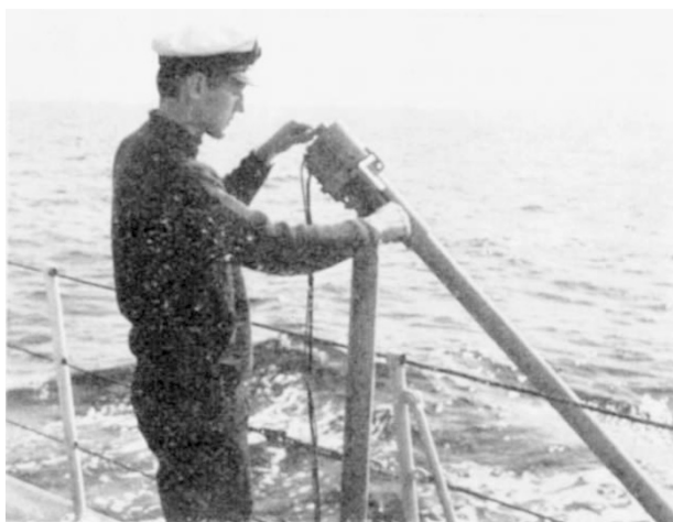
Preparing to fire a probe from the launcher unit of the expendable bathythermograph system.
