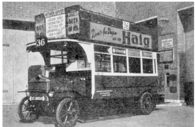
Two of the exhibits at Clapham. Locomotive No. 3 of the Furness Railway Co., delivered to the railway in 1849 and withdrawn from service in 1898; and a K-type omnibus of the London General Omnibus Co., 1919—the first design to have the driver seated beside the engine.
