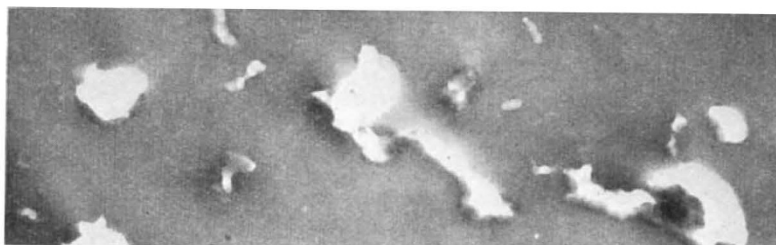
Fig. 1. Part of a thin section through A.C.I. C (sodium form). Membrane embedded in 'Epon 812' and sectioned with a glass knife. ( \times c. 16,700 )
