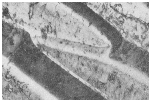
Fig. 1. A typical area of hot-worked graphite showing basal cleavage (x c. 265).
