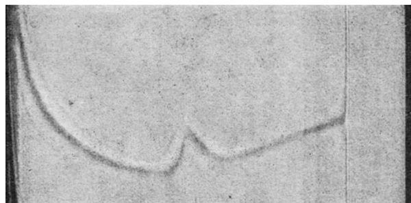
Fig. 1. Sedimentation diagram of renatured \alpha 1 after 18-h pepsin treatment; concentration prior to pepsin addition 2.6 mg collagen/ml. in 0.25 M citrate buffer, pH 3.7; temp., 22°; 59,000 r.p.m.; phase angle, 66°; photographed after 150 min
