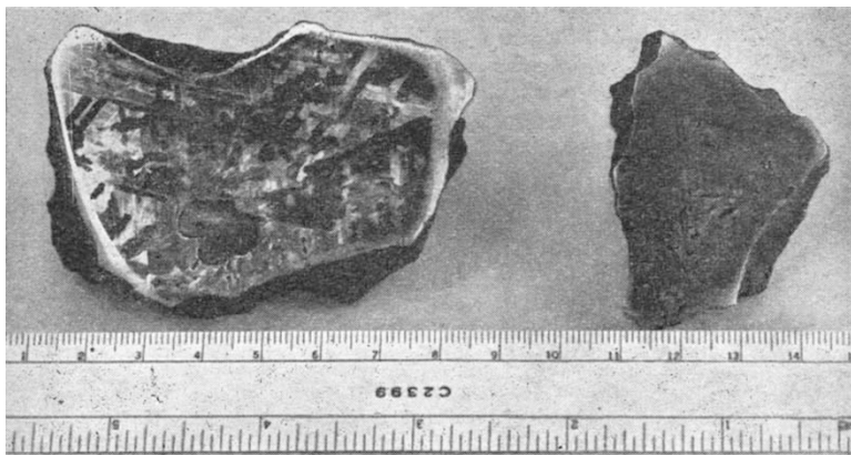
Fig. 1. Comparison between the apparently normal, undeformed Widmannstätten pattern of the moderately shocked Canyon Diablo No. 3 sample (left) with the faint deformed pattern of the heavily shocked Canyon Diablo No. 2 (right). The white areas on the polished surface of the Canyon Diablo No. 3 are \epsilon iron
