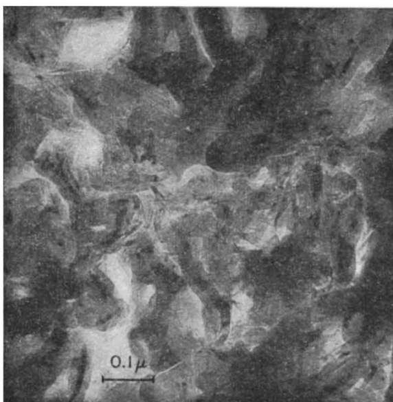
Fig. 1. Electron micrograph of an ultra-thin section of an apparent vitrain band in a meta-anthracite from Leoben, Austria. ( \times 93,750 ) (Unoriented section)
