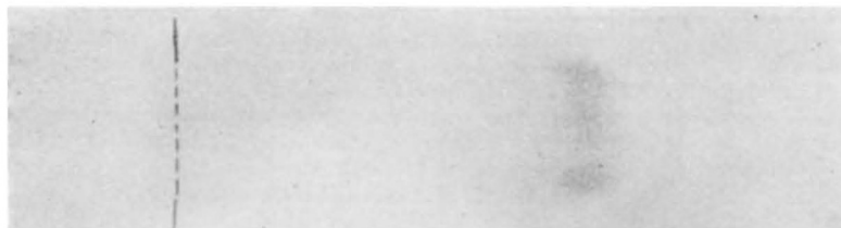
Fig. 1. The migration of serum albumin heated with congo red at (pH 6.4). The photograph was taken using a red filter to remove the red colour of congo on the strip
