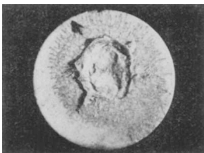
Fig. 5. Electrical porcelain after 10 shocks at 400 cal./cm.²sec.
