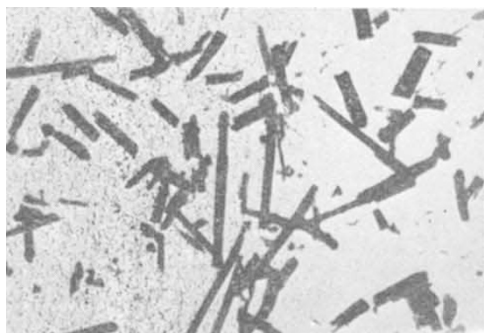
Fig. 2. Precipitates formed in an Fe-3 per cent Si alloy after nitriding and furnace cooling from 640°C, and then further annealing at 820°C. Extraction replica. (Electron micrograph \times 2,000 )
