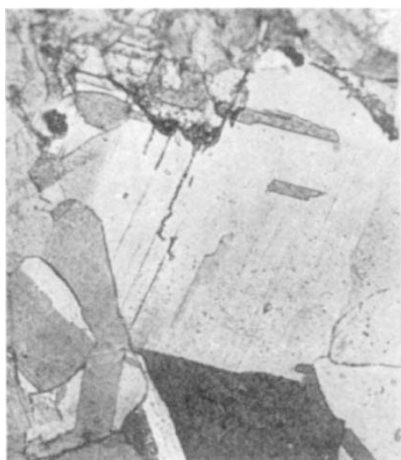
Fig. 2. Cross-section of the surface of a machined rotating-cantilever specimen of copper, showing short fatigue cracks running along striations. Specimen had fractured completely some 3 mm. from this point at 18,000 lb./sq. in. after 476,000 cycles at 170 c./min. Specimen axis horizontal. Etched with acid ferric chloride. \times 370
