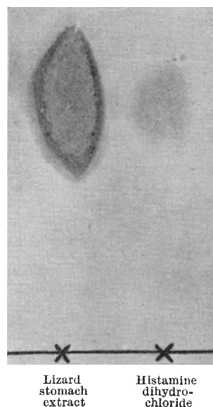
Fig. 1. Chromatogram of lizard stomach extract compared with histamine dihydrochloride, with propyl alcohol-acetic acid-water solvent
