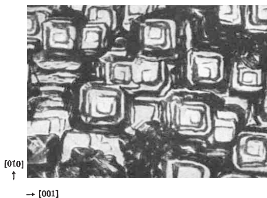
Fig. 1. Growth spirals in copper electrodeposited from an acid copper sulphate bath. ( \times 570 )
