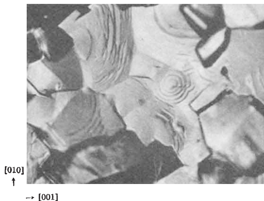
Fig. 2. A growth spiral in copper electrodeposited from a neutral copper sulphate bath. ( \times 940 )
