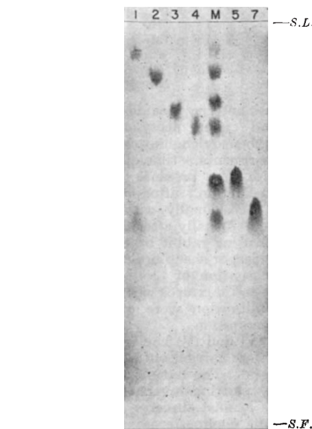
Fig. 1. Resolution of a mixture (M, above) of conjugates 1, 2, 3, 4, 5 and 7 using system III. Running time, 5½ hr. at 30.5°–32.5° C. S.L. designates starting line and S.F. solvent front
