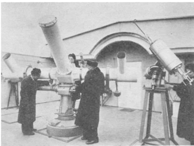
Fig. 3. The Linnik interferometer for measuring the separation of double stars. Academician Linnik is in the centre of the picture
