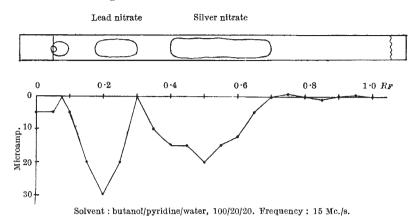
We have investigated the use of frequencies from 500 to 15,000 kc./s. and have found that the lower frequencies (500-5,000 kc./s.) promote greater sensitivity than the higher. We also find that each substance has an optimum frequency for maximum sensitivity. Further work is in progress in this direction.
