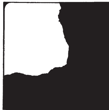
Corner of copper grid, cleaned by flaming. ( \times 2,700 )
