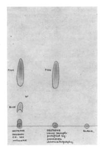
chromatograms, run before and after purification by our technique, showed that the impurity was completely removed by this means (see photograph).
