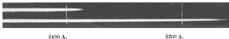
Hexamethylbenzene photographed through a calcite rhomb. The upper beam is polarized in the molecular plane, the lower perpendicular to it
