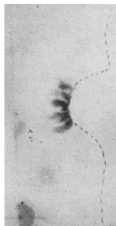
Fig. 3. Photograph of chromatogram obtained with 'Tween 80' and hæmin in the absence of any proteins. Solvent in both directions, M /100-fructose. Similar results are obtained with other combinations of solvents
