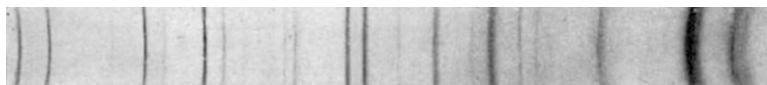
Debye-Scherrer pattern of gold wire taken with gallium K\alpha + \beta -radiation in 9-cm. diameter camera. Exposure 60 m.amp., 40 kVp., 1\frac{1}{2} min.
