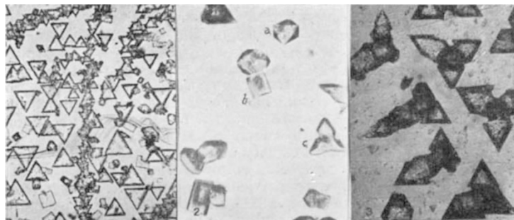
(1) Rubidium iodide crystals grown on mica. (2) Rubidium iodide crystals grown on a three-molecule layer of barium stearate deposited on mica, showing the development of hexagonal outlines (a), an unoriented cubic crystal (b), and a connected group of three (c). (3) Connected groups of three crystals growing on a monolayer of barium stearate on mica. In each photograph the longest side is parallel to the b -axis of the mica, and the magnification \times 80
