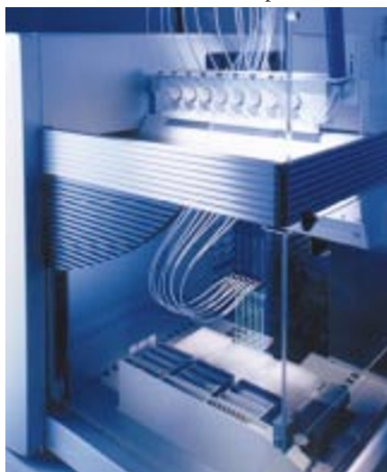
Let there be blue light: the GENESIS Workstation tackles volumes down to 0.5 µl.
