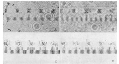
(B) shows a direct reconstruction from the original hologram (A) using the technique previously described without any intervening auxiliary lens. It is, in fact, a particular Fresnel diffraction pattern of A. (D) is a similar reconstruction from (C). It will be seen at once that (B) bears a close resemblance to the original microscope scale, as anticipated, and (D) bears a more distant but still recognizable relationship.
