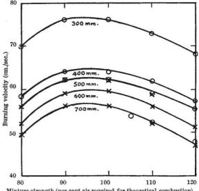
Mixture strength (per cent air required for theoretical combustion) -x-, Burner diam. 1.0 cm.; 0-0-, burner diam. 1.27 cm.
