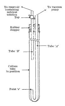
The working principle of the apparatus is as follows: a culture tube is placed in position and liquid is run in via tube B; the level of the liquid rises until it reaches the top of the short arm e, when any surplus is drawn off via tube A. It is the height of e which predetermines the volume of liquid remaining in the culture tube (assuming a fairly high degree of uniformity in the culture vessels in use).
