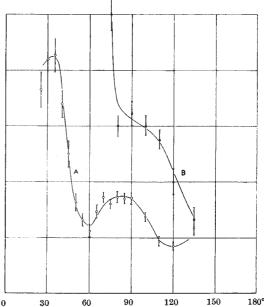
Angular variation of intensity of deuterons scattered inelastically (curve A) and elastically (curve B) from magnesium
