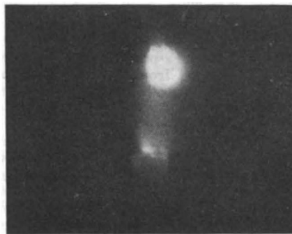
Bright region in the neighbourhood of the cathode of a high-pressure mercury-vapour discharge showing intense barium spectrum
