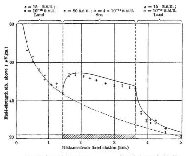
, Theoretical curve, land and sea; — · — · —, theoretical curve, land only; +, measurements at fixed station; o, measurements at mobile station.  $\lambda = 3.9 \text{ m.}$ ; P = 10 watts; vertical polarization,  $h_T = h_R = 0$
