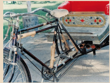
Inappropriate technology: 'regenerative' brakes on rickshaws ignored the cost of retrofitting
