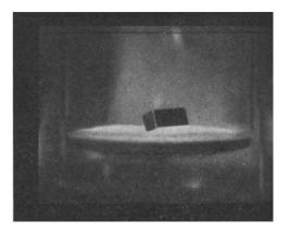
disk 40 mm, in diameter in a Dewar vessel over liquid helium.
