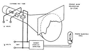
In addition to the applications mentioned by Mr. MacKay, it is possible to combine a pair of electronic function generators to form a high-speed electronic analogue multiplying unit. This aspect has been dealt with in an article which was accepted for publication<sup>3</sup> towards the end of 1946.
