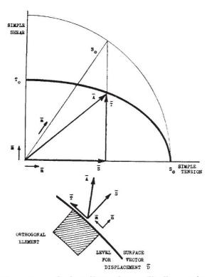
Such a linear form will allow easier stress case. analysis of many particular cases arising from the application of my theory of post-yield stress-strain<sup>5</sup>. In that theory the Huber criterion was used to give the simple tensile stress 'corresponding' to the complex stresses operating at any point in the yielded field. The new linear criterion can be used in the same way.
