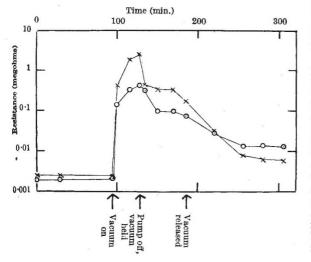
These observations suggest that the current path in moist wood is principally along the interior surfaces of the cells. If the current path were through the body of the cell walls, the sudden drying of the interior surfaces on evacuation could only cause an insignificant increase in the average resistance, whereas the observed resistance increases between one and two hundred times.
