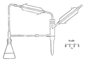
The condensed water is washed into the receiver by succeeding portions of liquid, whilst the return flow takes place through a lower connecting tube. The second condenser is introduced to prevent any loss of solvent. Connexions are made by synthetic rubber ('Neoprene') tubing, which is resistant to organic solvents, across butt-end glass joints. We are indebted to Mr. L. G. Wilkinson for the construction of this apparatus.
