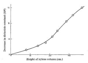
Changes in the dielectric constant during flow are observed in polar as well as in non-polar liquids. But a more viscous liquid like amyl alcohol is found to show the effect to a much smaller degree. Observations with liquid heights greater than that shown in the graph could not be taken due to certain practical difficulties. Further investigations are, however, in progress and a detailed report will be published elsewhere.
