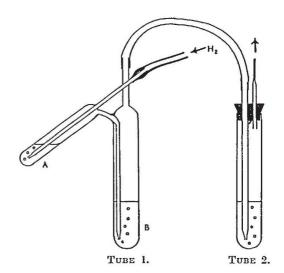
The apparatus used is shown in the accompanying diagram. Five c.c. of a 0.1 per cent solution of hydrogen peroxide in 0.125~M phosphate buffer,  $p{\rm H}$  7.3, and 0.25~M sodium chloride were introduced into the rear arm (A) of tube 1, which was then connected by lead tubing to a heavy glass tube containing palladium asbestos. The glass to lead connexions were sealed with de Khotinsky cement.
