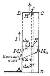
force at any distance x from AB and remote from BC or AD is H = 2I/x + 2I/(b-x), and hence if the length of the loop is increased by the amount dy
