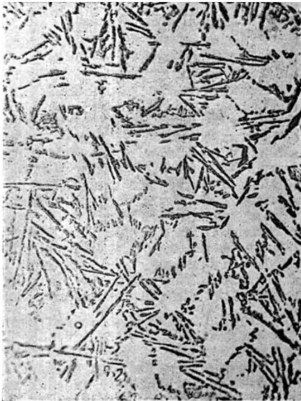
FIG. 1.—9.86 per cent. Si, 0.45 per cent. Fe. Chill cast. Unetched. \times 200 .
