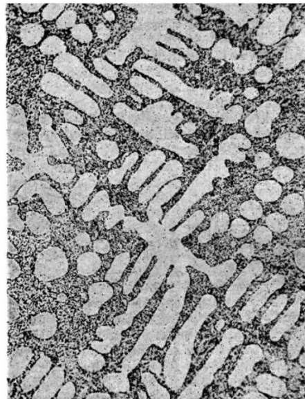
FIG. 2.—9.86 per cent. Si, 0.45 per cent. Fe. Same alloy as Fig. 1, but modified with 5 per cent. NaOH at 750^{\circ}\text{C} . Chill cast. Etch HF. \times 200 .
