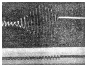
damped coupled vibration of the string and bridge, in many respects differing from the cyclical vibrations excited by bowing at the "wolf-note" pitch described by me in previous communications to NATURE. At pitches slightly different from that of the "wolf-note," the dissipation of energy is far less rapid, and the motion of the string approximates to that of an ordinary damped harmonic vibration.
