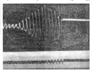
damped *coupled* vibration of the string and bridge, in many respects differing from the cyclical vibrations excited by *bowing* at the "wolf-note" pitch described by me in previous communications to NATURE. At pitches slightly different from that of the "wolf-note," the dissipation of energy is far less rapid, and the motion of the string approximates to that of an ordinary damped harmonic vibration. C. V. RAMAN.
